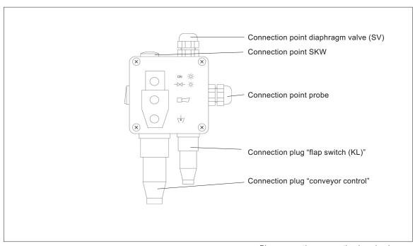
Plug connection connection housing hopper
